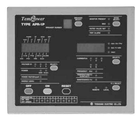
The operation panel, which is an integrated monitoring and control tool, has functions and capabilities of watt-hour meters, wattmeters, voltmeters, ammeters, switches, and indicators, allowing the operator to remotely monitor and control up to eight ACBs via serial communications.
